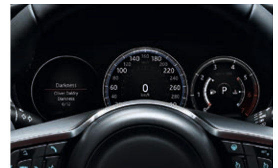
12.3" Full Digital Instrument Panel with virtual dials
